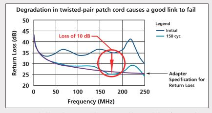
As you can see in this graph, a commercial Cat 7 SSTP cord has a 10 dB loss after 150 cycles of coiling and uncoiling. This 10 dB degradation causes a good link to fail – and you end up with a false fail. This 10 dB of loss won't occur when you use Fluke Networks' Permanent Link adapter technology – with DTX you get repeatable accuracy you can count on.
